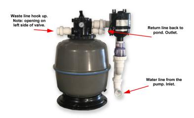
Make plumbing hook ups as shown in the picture. For your convenience the UniClears come with unions for easy access to the internals. Simply glue 2" pvc pipe into the unions and you're set.
