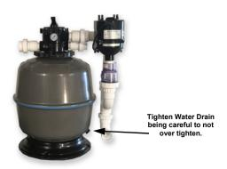
Some of the UniClear filters come with Media inside and ready to go and some require the installation of the media after arrival. Simply remove the multiport valve. Make sure the lateral assembly is centered on its resting pivot. Apply a piece of tape to cover the opening to the center pipe and then pour in the media. Remove the tape. Replace the multiport making sure the large O ring is still in place around the area just below the lip of the multiport. That's it, ready to
