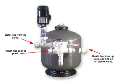
Make plumbing hook ups as shown in the picture. Use 2" pipe to connect to unions to secure plumbing to valve. For ease of use we recommend a 3 way valve be installed and water flowed to the PoliGlassBead when a polish of the water is needed and the rest of the time the water can be bypassed around the PoliGlassBead filter.
